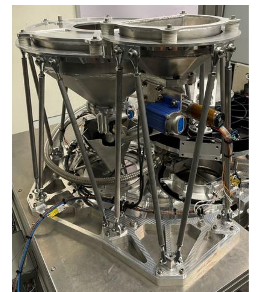
Carbothermal reduction hardware from Sierra Space (CaRD) and molten regolith electrolysis diagram
